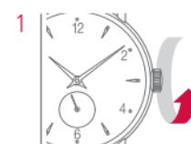
1 Rotate the crown carefully multiple times clockwise until you feel resistance.
