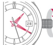
Move the crown counter-clockwise until the date changes. Then deliberately set the current time either a.m. or p.m.
