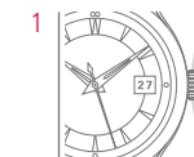
Manually wind the movement by rotating the crown at least 30 times in the clockwise direction.
