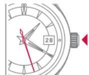
Push the crown back to the initial position. The second hand is back in motion.
