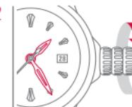
2 Move the crown counter-clockwise until the date changes. Then deliberately set the current time either a.m. or p.m.
