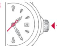
3 Push the crown back to the initial position. The second hand is back in motion.
