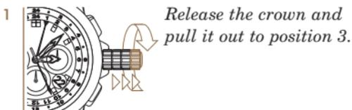
1 Release the crown and pull it out to position 3.
