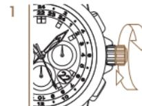
1 Rotating the crown in the counter clockwise direction will automatically release it to position 1.
