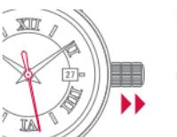
Pull the crown until it is in position 2. The second hand does not move.
