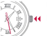
Push the crown back to the initial position. The second hand is back in motion.
