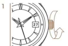
Manually wind the movement by rotating the crown at least 30 times in the clockwise direction.
