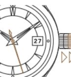
Pull the crown until it is in position 2. The second hand does not move.
