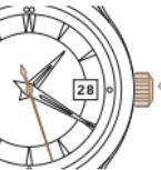
Push the crown back to the initial position. The second hand is back in motion.
