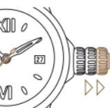
Pull the crown until it is in position 2. The second hand does not move.
