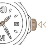
Push the crown back to the initial position. The second hand is back in motion.
