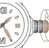
Move the crown counter-clockwise until the date changes. Then deliberately set the current time either a.m. or p.m.
