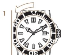
1 Rotate the bezel counter-clockwise.
