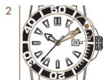
2 Set the marking on the bezel to the minute hand.
