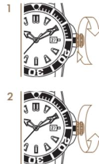
Rotating the crown in the counter clockwise direction will automatically release it to position 1.
