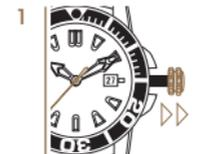
Pull the crown until it is in position 3. The second hand does not move.
