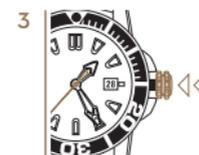
Push the crown back into position 1. The second hand is back in motion.
