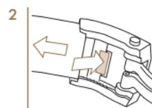
2 To lengthen the bracelet/strap, hold down the button and carefully move the bracelet/strap to the desired position.
