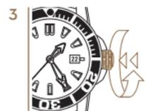
3 Press the crown against the case and simultaneously turn clockwise until it is firmly secured.
