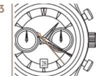
3 Read the average speed by optical extension of the seconds counter.
