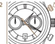
2 To stop measuring time, press the P1 pusher again. The seconds counter stops immediately.
