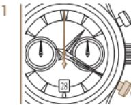
1 While time measurement is in progress, push the P2 pusher to reset all the counters to zero. The next time measurement starts automatically. In order to put all the counters back to zero after that, press the P2 pusher with the chronograph function stopped.
