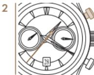
2 To stop measuring time, press the P1 pusher again and read where it stopped.
