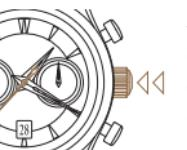
Push the crown back to the initial position. The second hand is back in motion.
