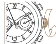
Manually wind the movement by rotating the crown at least 30 times in the clockwise direction.
