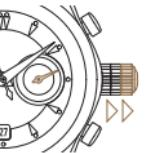
1 Pull the crown until it is in position 2. The second hand does not move.
