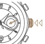
3 Push the crown back to the initial position. The second hand is back in motion.
