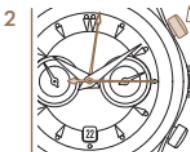
*To stop measuring time, press the P1 pusher again and read where it stopped.*
