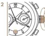
*Set the current date by rotating the crown counter-clockwise.*
