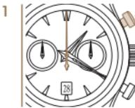
*Start the tachymeter function by using the P1 pusher. The seconds counter is in motion.*
