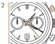
*To stop measuring time, press the P1 pusher again. The seconds counter stops immediately.*
