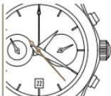
3 Read the average speed by optical extension of the seconds counter.
