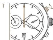
*Start measuring time using the P1 pusher. The seconds counter is in motion.*
