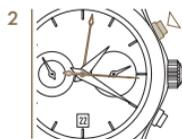
*To stop measuring time, press the P1 pusher again and read where it stopped.*
