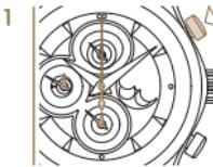
1 Start measuring time using the P1 pusher. The seconds counter is in motion.
