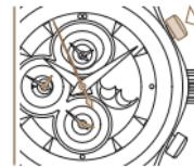
2 To stop measuring time, press the P1 pusher again and read where it stopped.
