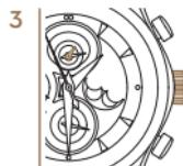
3 Push the crown back to the initial position. The small seconds hand is back in motion.
