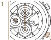
1 While time measurement is in progress, push the P2 pusher to reset all the counters to zero. The next time measurement starts automatically. In order to put all the counters back to zero after that, press the P2 pusher with the chronograph function stopped.
