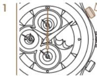
1 Start the tachymeter function by using the P1 pusher. The seconds counter is in motion.
