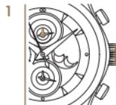
1 Pull the crown until it is in position 1. The small seconds hand does not move.
