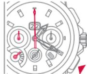
While time measurement is in progress, push the **P2** pusher to reset all the counters to zero. The next time measurement starts automatically. In order to put all the counters back to zero after that, press the **P2** pusher with the chronograph function stopped.
