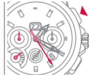
Start measuring time using the **P1** pusher. The seconds counter is in motion.
