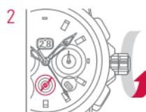
Rotate the crown clockwise until the power reserve indication hand has left the red area.
