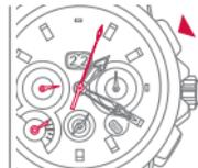
To stop measuring time, press the **P1** pusher again and read where it stopped.
