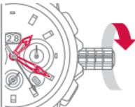
Move the crown counter-clockwise until the date changes. Then deliberately set the current time either a.m. or p.m.
