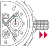
Pull the crown until it is in position **3**. The second hand does not move.
