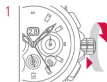
Rotating the crown in the counter clockwise direction will automatically release it to position 1.
