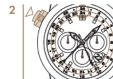
2 Press the monopusher repeatedly until the 24 on the rotatable scale is under the 24 on the fixed scale.
