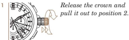
1 Release the crown and pull it out to position 2.
