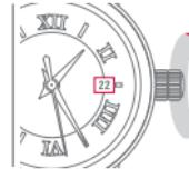
2 Set the current date by rotating the crown counter-clockwise.
