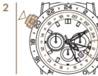
*Press the monopusher according to the number of time zones (five in this example) and then push it back to its neutral position.*
