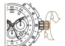
*Rotating the crown in the counter clockwise direction will automatically release it to position 1.*
