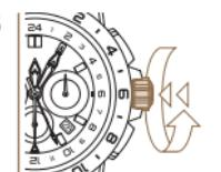
*Press the crown against the case and simultaneously turn clockwise until it is firmly secured.*
