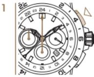
*Start measuring time using the P1 pusher. The seconds counter is in motion.*
