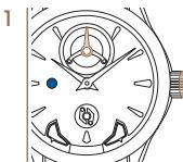
*Pull the crown into position 1 as far as it will go. The second hand stops, along with the tourbillon cage.*
