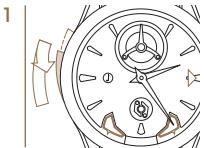
*Push the minute repeater activation lever down and release it again. As long as the time is acoustically indicated, the crown cannot be pulled out.*
