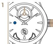
*Pull the crown into position 1 as far as it will go. The second hand stops, along with the tourbillon cage.*
