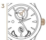
*Push the crown back to the starting position. The second hand and the tourbillon cage start moving again.*
