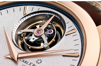
The tourbillon is considered another major highlight of the watchmaker's craft, and compensates for the variances caused by the works of a mechanical watch. Due to the different positions of the watch on the wrist, the earth's gravity influences the movement of the balance at any given time.
