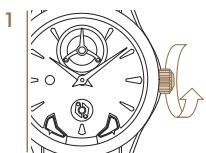
*Manually wind the movement by rotating the crown at least 30 times in the clockwise direction.*
