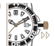
*Pull the crown until it is in position 3. The second hand does not move.*
