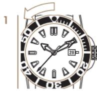
1 Rotate the bezel counter-clockwise.
