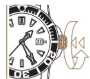
3 Press the crown against the case and simultaneously turn clockwise until it is firmly secured.
