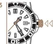
*Push the crown back into position 1. The second hand is back in motion.*
