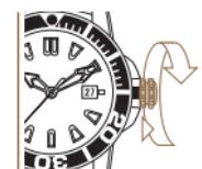
*Rotating the crown in the counter clockwise direction will automatically release it to position 1.*
