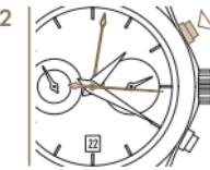
2 To stop measuring time, press the P1 pusher again and read where it stopped.
