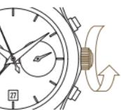
Manually wind the movement by rotating the crown at least 30 times in the clockwise direction.
