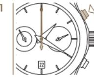
1 Start measuring time using the P1 pusher. The seconds counter is in motion.
