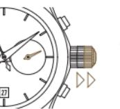
Pull the crown until it is in position 2. The second hand does not move.
