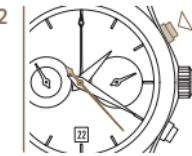
2 To stop measuring time, press the P1 pusher again. The seconds counter stops immediately.
