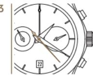
3 Read the average speed by optical extension of the seconds counter.
