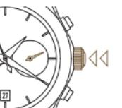
Push the crown back to the initial position. The second hand is back in motion.
