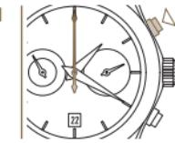
1 Start the tachymeter function by using the P1 pusher. The seconds counter is in motion.
