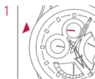
1 Use a corrector pin to press corrector **A** repeatedly until the hand is on the desired hour.
