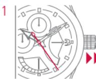
1 Pull the crown until it is in position **2**. The second hand does not move.
