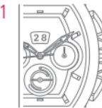
Rotating the crown in the counter clockwise direction will automatically release it to position 1.
