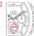
Rotate the crown clockwise until the power reserve indication hand has left the red area.
