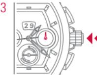
3 Push the crown back into position **1**. The second hand is back in motion.
